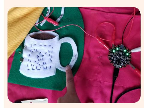
You may use any conductive material to act as your button, such as a metal button, aluminum foil, copper tape, or anything else conductive. It just needs to be securely connected back to the CPX with conductive thread.
