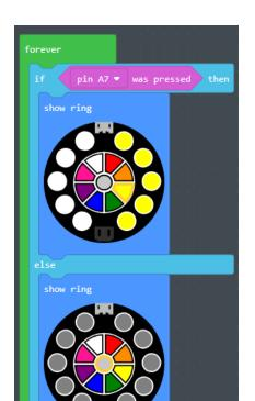
We need a trigger to begin this program, so go into the LOOPS section and bring out the FOREVER block, wrapping around the other blocks.
